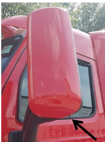
FIGURE 1-8. Aerodynamic Mirror OAT Sensor Location
